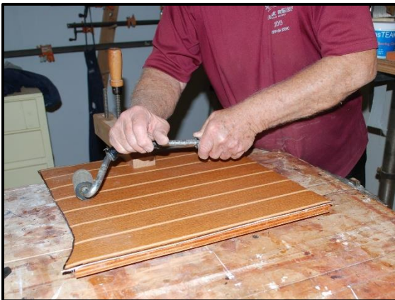
Figure 8 Pressing the Vinyl with Laminate Roller
