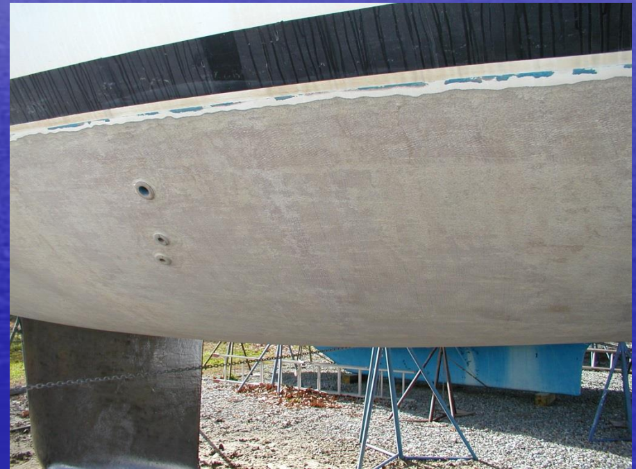
This part of the hull has been completely sandblasted
